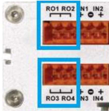
**R01:** Relay #1 from ICP pins 11 & 29 move to the Barix upper left connector pins 1 & 2 – Local Break Start
