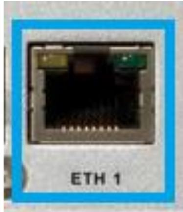
On the front panel, normally the green LED is solid with a blink every three seconds. The red LED will illuminate and blink during booting of the unit, but once the unit has booted if the red LED stays on or is blinking, it indicates a problem locking onto the audio stream and/or with the unit configuration.
