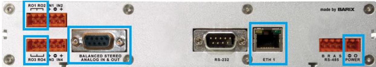
Connect the provided audio breakout cable to the rear panel **Balanced Stereo Analog IN & Out** connector. This breakout cable ships to you with screw terminal adapters for the audio connections, no soldering of audio connectors is needed.
